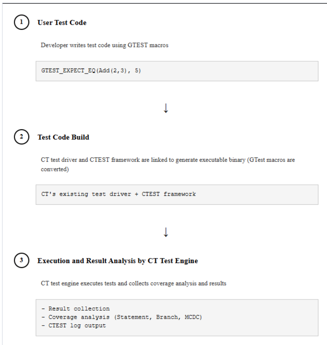
Figure 1 Code-Based Test Execution Flow
